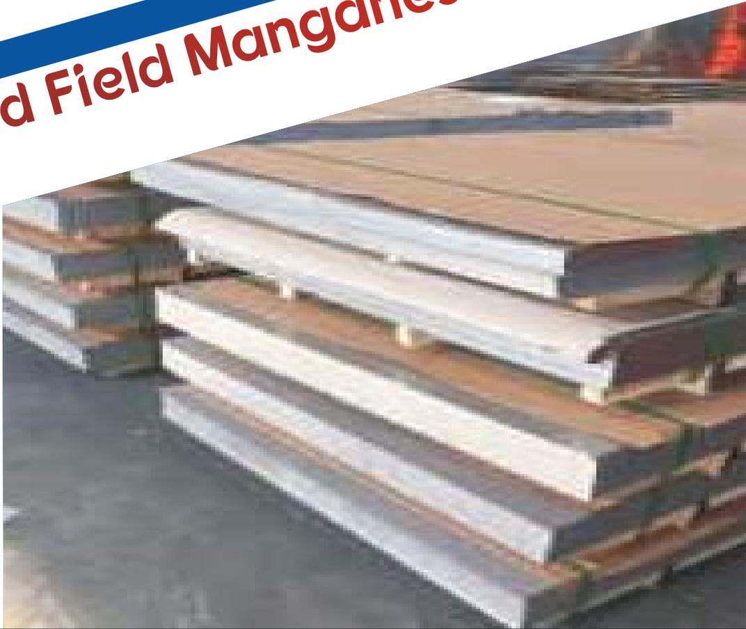
Widely known for its work hardening properties, **Hardfield Manganese Steel Plates** are amenable to high-impact wear applications or those in which scratch abrasion is encountered. These hardened steel plates enhances almost five times the hardness of mild steel and almost three times the hardness of annealed stainless steel. Due to this, one can enjoy a longer lifespan and extended protection of their equipment and facilities.
